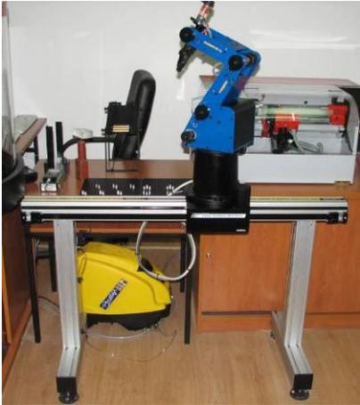
Figure 12: Floor-Mounted Linear Slidebase
