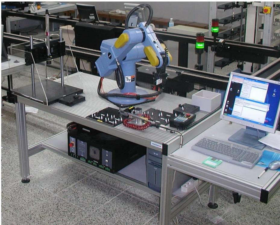
Figure 59: Pneumatic Press Station with SCORBOT ER-9Pro
