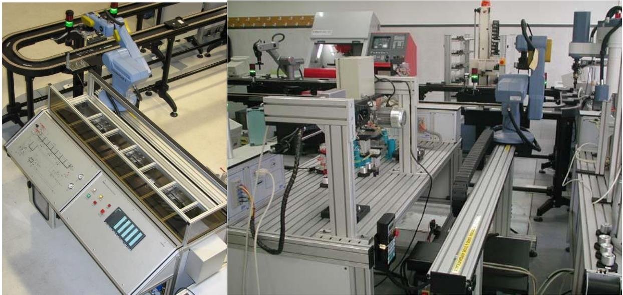
Figure 60 and 20: Process Station and Mechatronic Station with SCORBOT ER-9
