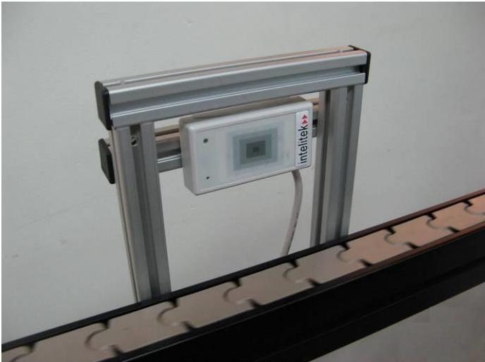
Figure 32: RFID System
