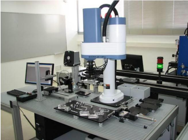
Figure 49: Assembly Station with SCORA ER-14
