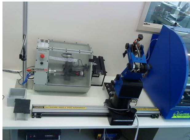
Figure 13: Table-Mounted Linear Slidebase
