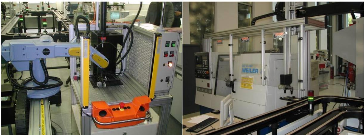
Figure 21 and 22: Industrial Hydraulic Press Station with SCORBOT ER-9Pro and Cartesian MTS Loader
