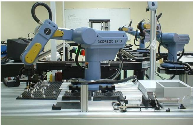
Figure 50: Assembly Station with SCORBOT ER-9
