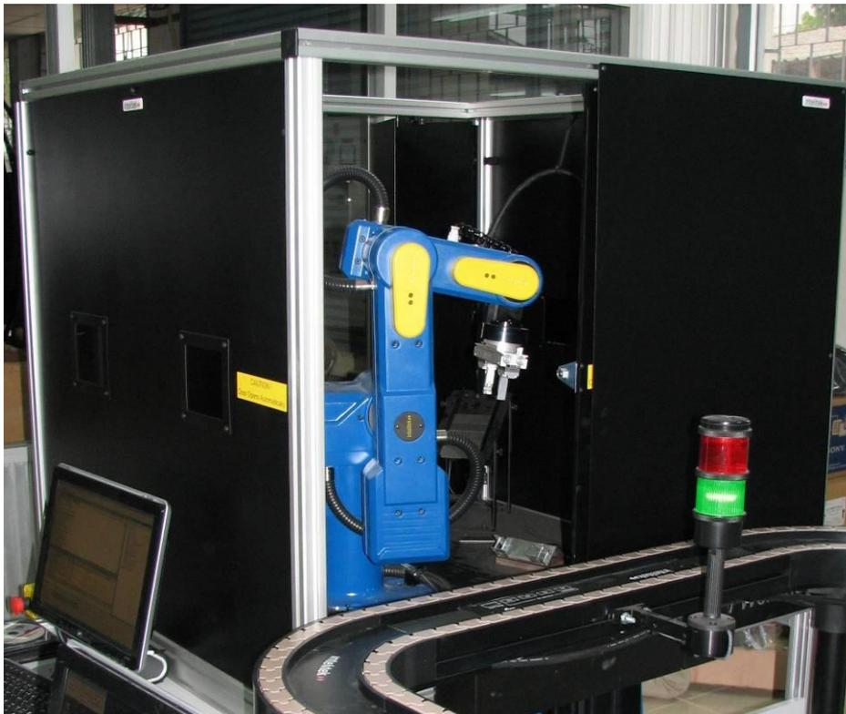
Figure 55: Welding Station with SCORBOT ER-9
