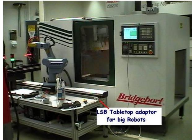
Figure 15: Table-Mounted Linear Slidebase
