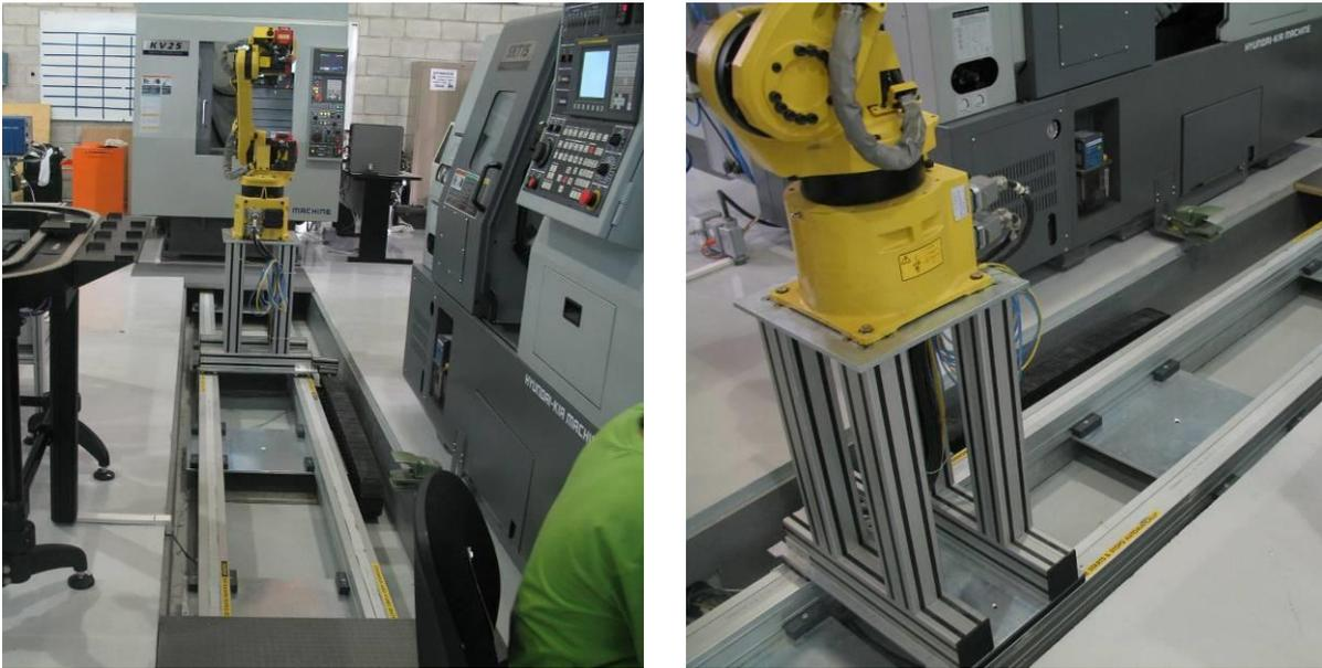
Figure 17: XtraDrive Linear Slide Base – Type 2
