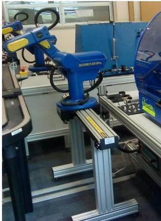
Figure 14: Floor-Mounted Linear Slidebase
