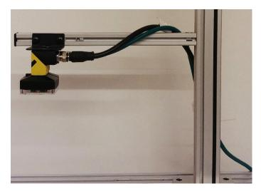
**4.** Secure the loose sections of the cables to the table using cable clamps and nylon cable ties. The clamps should be secured to a slotted table with M5 flat head Allen screws and T-slot nuts, and to a Formica table with pan head Phillips screws.
