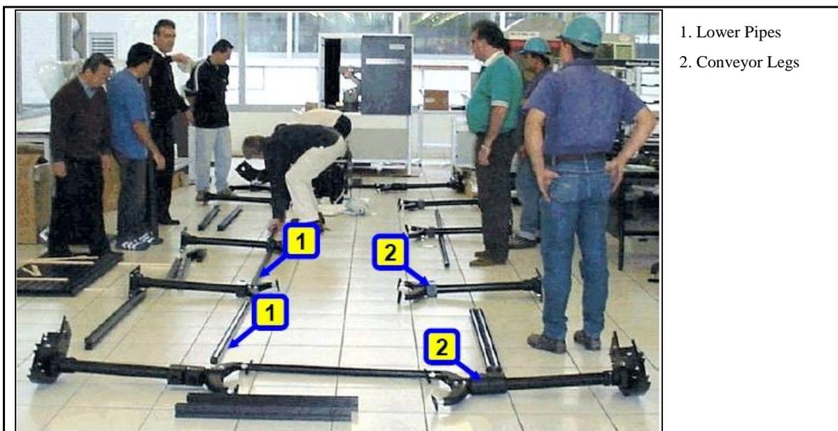
Figure 2: Conveyor Components – Floor Layout
