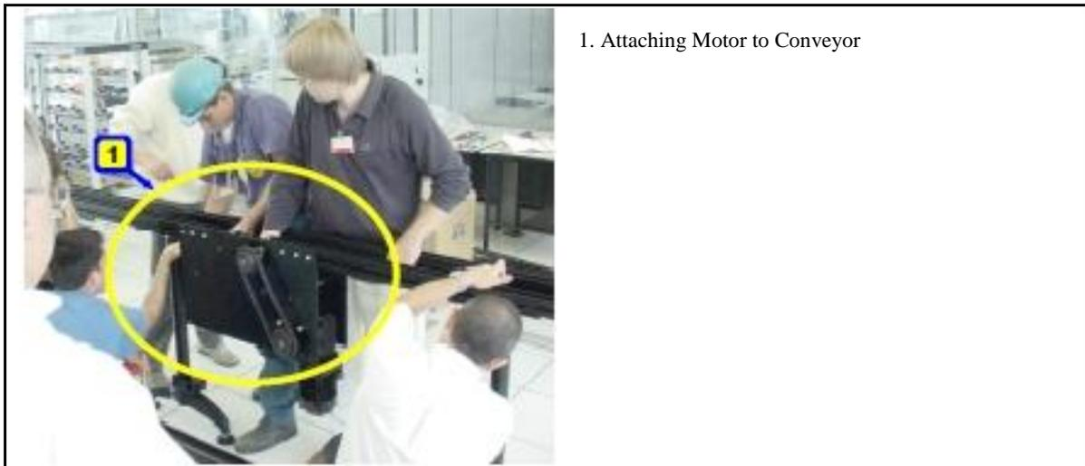
Figure 11: Lifting Motor into Conveyor Gap
