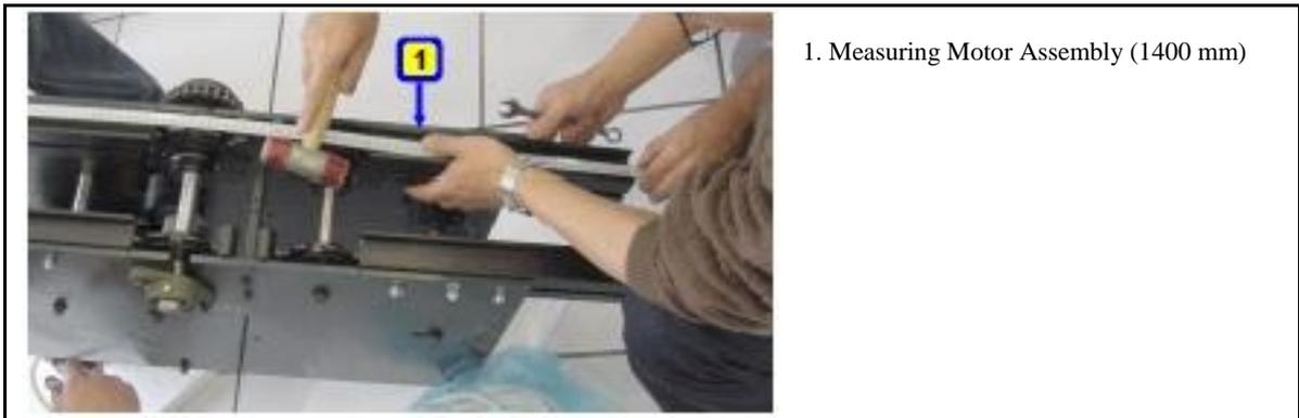
Figure 10: Fine Tuning the Motor Unit
