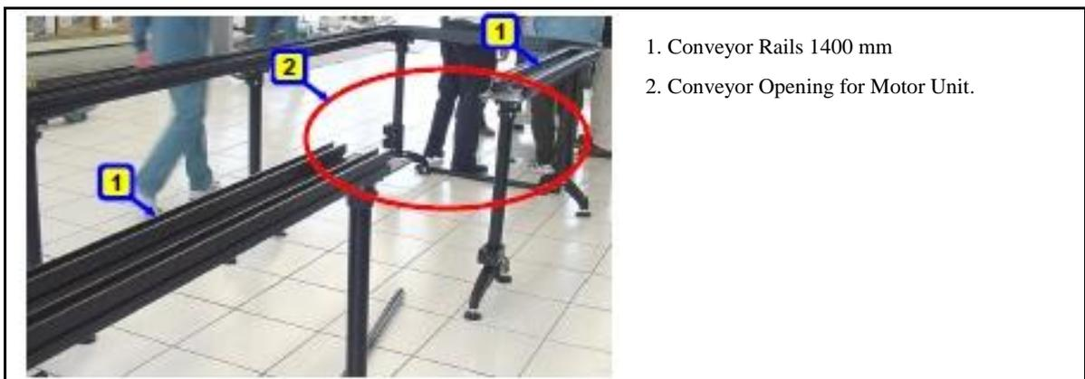
Figure 7: Conveyor Opening for Motor Unit
