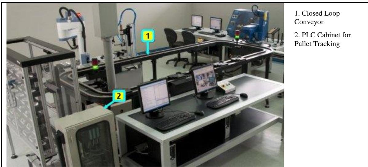
Figure 1: Closed Loop Conveyor
