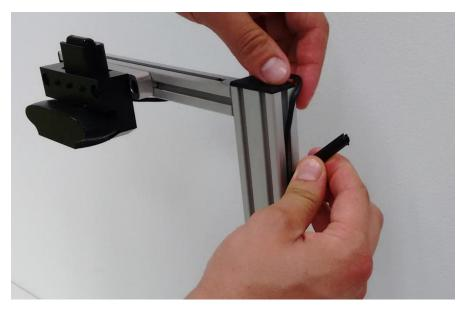
8. Secure the remainder of the wire to the table using cable clamps and nylon cable ties. The clamps should be secured to a slotted table with M5 flat head Allen screws and T-slot nuts, and to a Formica table with pan head Phillips screws.
