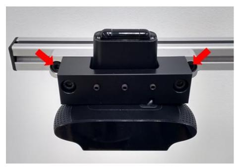
**6.** Tighten the three small Allen screws of the camera holder. These screws further stabilize the camera, preventing it from wobbling.
