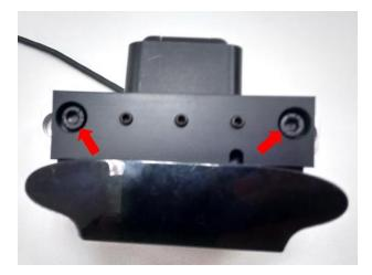
**4.** On the support side of the assembly, screw in a 1/4 inch Allen screw.
