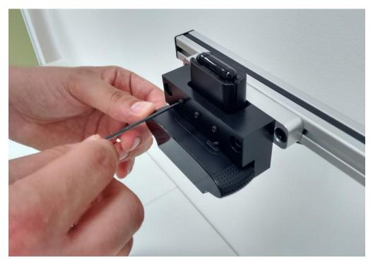
① Note: You must ensure that the camera is not free to move once attached.
