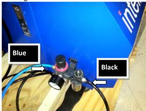
4. Connect the blue air hose to the building's air supply using the T-fitting supplied in the kit.
