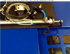
4. Connect the black air supply hose to the available receptacle on the solenoid valve.
