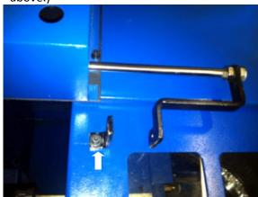
10. Use the socket head cap screw removed in step 8 above to attach the "L" bracket to the piston bracket, and tighten securely.
