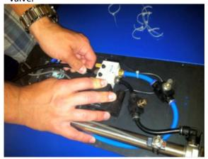
5. Route the black hose and the control wires from the air shield assembly through the holes on the assembly's cover as shown.
