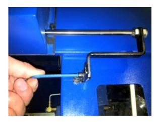
11. Tighten the seven screws around the assembly to secure the assembly to the enclosure.
