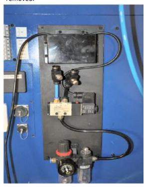
3. Connect the blue tubing from the shield opener to the blue output on the pneumatic panel, and the black tubing to the black output. You may cut the tubing to length using a tubing cutter.
