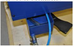
2. Tighten the tubing clamp over the barb fitting.
