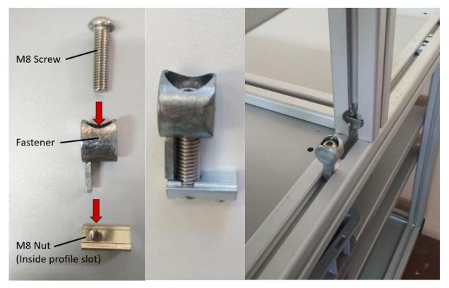
c. Push the screw/fastener/nut assembly into the circular pocket of the working surface's leg.
