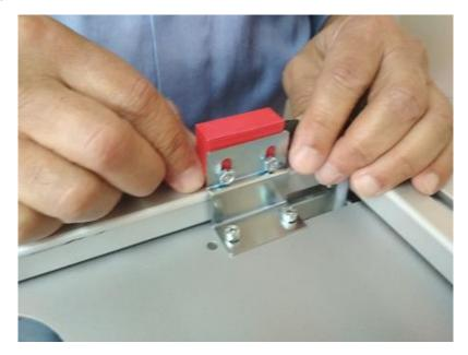
**4.** Place the safety guard assembly on top of the working surface. Ensure that the two read heads are touching and aligned. If they are not, remove the safety guard and adjust the height of the read head connected to the controller. Replace the safety guard to confirm alignment.
