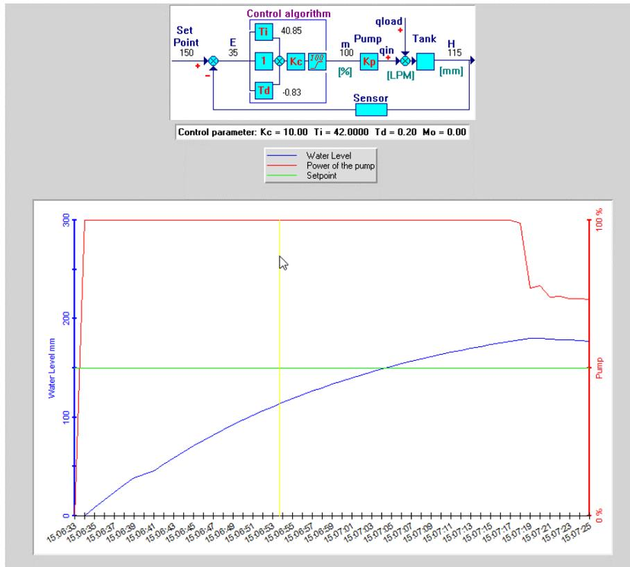
**Graph of a stopped process with a vertical yellow line. Values of the responses intersected by the yellow line represent the values at the indicated point of time. The values are displayed in the Block Diagram above the graph.**
