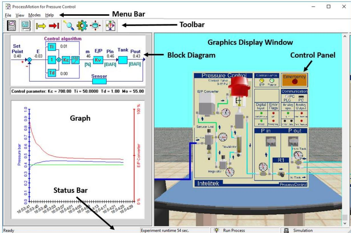
Initially, before a process is started, the Block Diagram and Graph areas are hidden.
