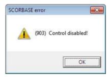
When SCORBASE is in Off-Line mode, the Control state cannot be altered.
