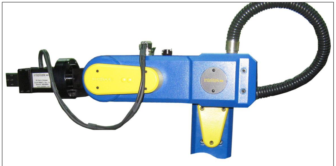
Figura 4-14: Conectar la pinza a SCORBOT-ER 9Pro
