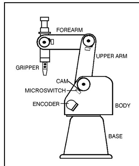
*Figure 2: Robot Arm Parts*
