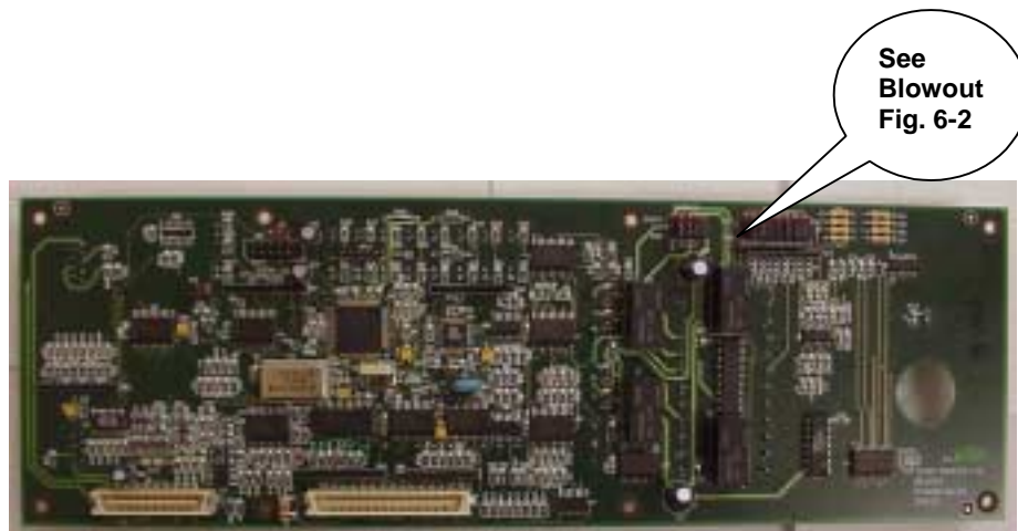
Figure 6-1 Jumpers Location
