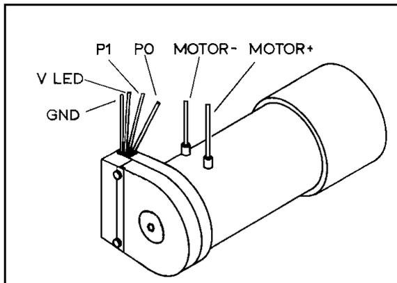
Figure 25: Motor Wiring
