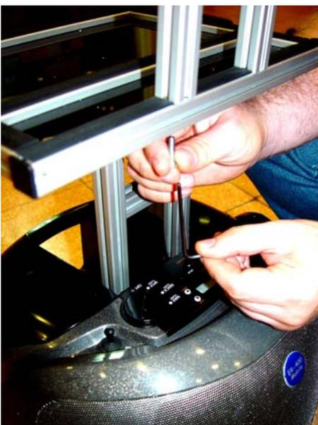
Attach the Payload Shelf supports to the top of the on-board PC shelf using the two M5x20 Allen screws provided. The Payload Shelf itself comes already assembled with its two vertical supports. The screws must be driven with an Allen wrench. Hold the Allen wrench as shown, using only the short end to tighten the screws. Be careful to avoid overtightening.
