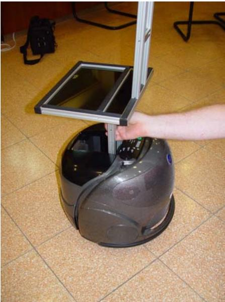
2. The AGV may be lifted and moved using the handle portion of the payload stand, as shown in the illustration. This is the safest way to move the AGV without using its motors.
