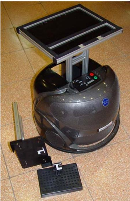
The ER-400 comes with a specially-engineered stand to support an on-board laptop computer and a payload. The stand includes a horizontal crossbar to be used as a handle for lifting, a large shelf for the laptop computer, and a small shelf for the payload.
