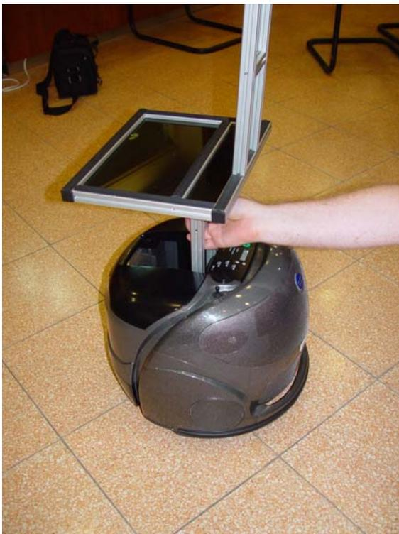
4. Gently lift the Mobile Robot out of the carton. Use only the aluminum lifting handle to support the weight of the Mobile Robot. Do not put any pressure on the Bumper Guard (also called Bumper or Bump Sensor), which occupies most of the front of the unit. See page 6 for a diagram identifying the parts.
