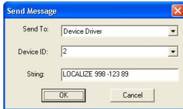
Once the Mobile Robot has thus been instructed as to its actual location, it can be directed to move to its originally intended destination by means of running a docking path. See page 25.
