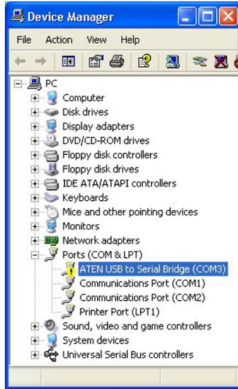
On the on-board PC, open the Control Panel. Click on the System icon to access the System Properties dialog box. Click on the Hardware tab. In the Device Manager subpanel, click the button for Device Manager. This opens up a directory tree. Select the node that reads PORTS and open it. Take note of the COM port number that has been assigned to the ATEN USB to Serial Bridge.
